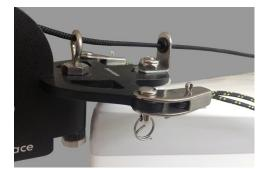
• These last 2 pictures illustrate the finished product. If done correctly, the foot-pedals on your footbrace should not need any adjustment when you move from under-stern steering to over-stern steering as the adaptor post keeps the rudder lines in the same position.
